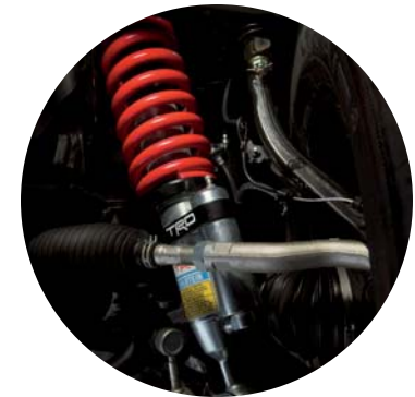
TRD Pro Bilstein® shocks with remote reservoirs
